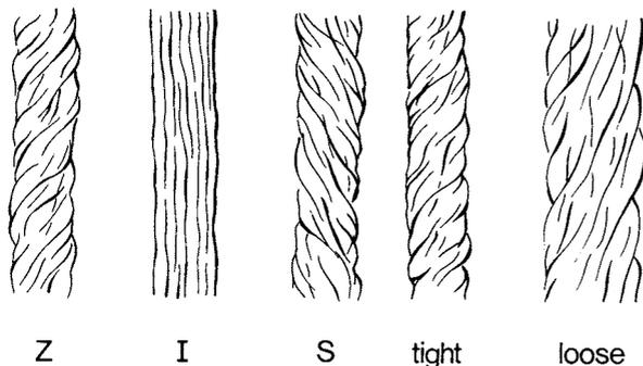
Fig. 124 The lie of fibres in a yarn
