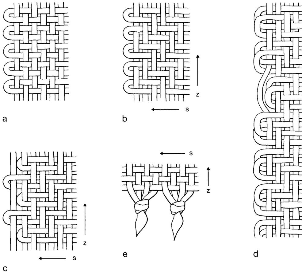
Fig. 127 Selvedges: a, simple, on tabby weave, e.g. 1260; b, on 2/2 chevron twill, 1306; c, on 2/2 chevron twill 1303; d, on diamond twill, 1382; e, fringe on wool textile in tabby weave, 1257. Not to scale.
