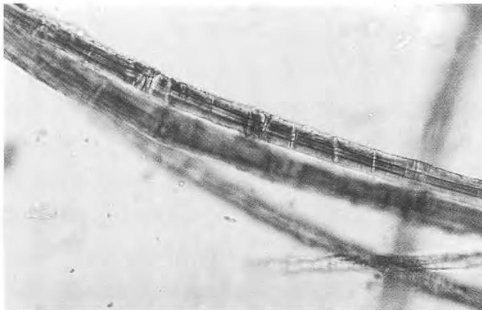
*Plate XVb* Photomicrograph of flax fibres from 1445; photographed at  $\times 400$
