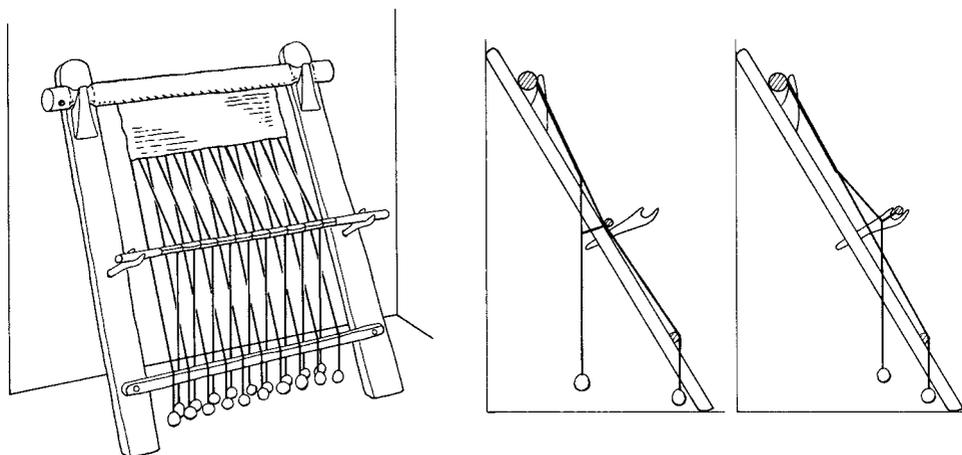
Fig. 139 Weaving tabby on the warp-weighted loom
