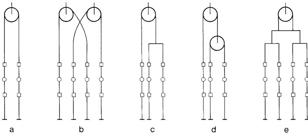
Fig. 163 Possible treadle-heddle-pulley tie-ups for the horizontal loom. Tabby may be woven with the tie-up shown in a; 2/2 twill with b; 2/1 twill with c and d; striped tabby, 1417, with e (and see Fig. 161)
