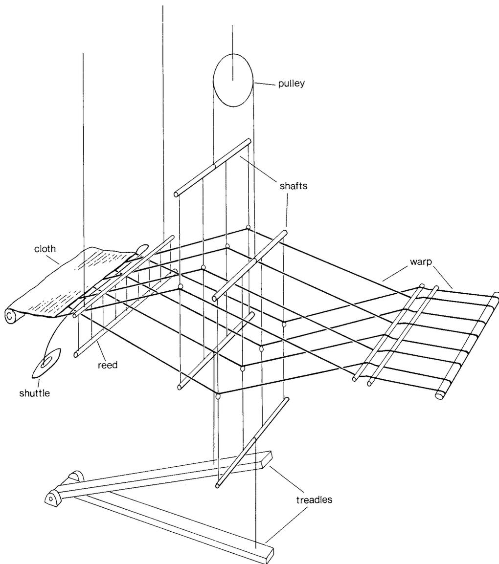
Fig. 162 *The horizontal loom*
